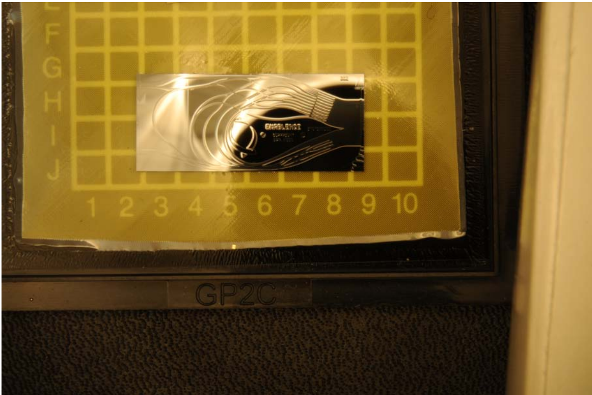
Fig. 3. A optical circuit for use in a custom biophotonic application.
