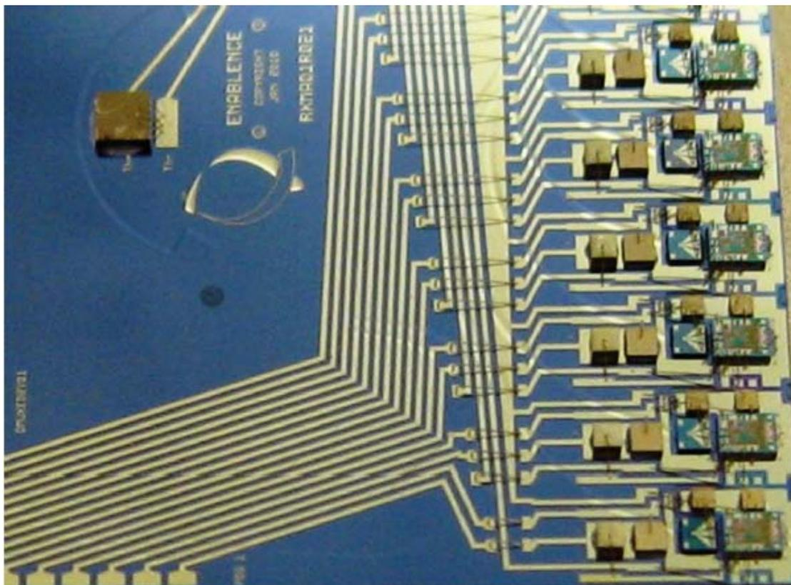
*Fig. 2. Close-up view of a Planar Lightwave Circuit that integrates WDM functionality, along with hybrid receiver photodiodes, transimpedance amplifiers, capacitors, thermistors, and other sub-components on a silicon chip.*
