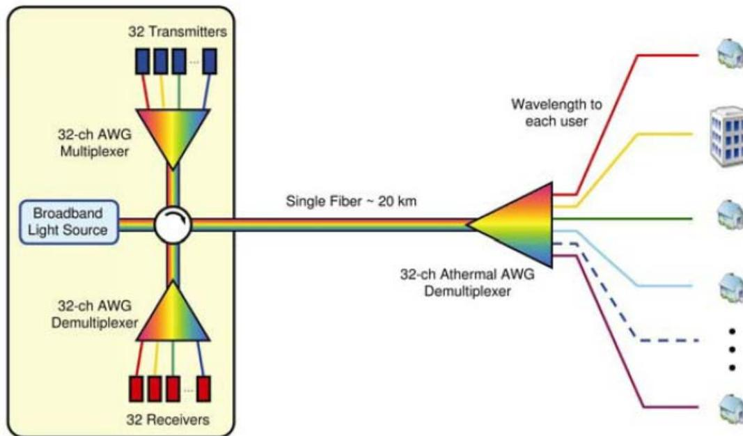
*Fig1: Schematic representation of a simplified WDM-PON system.*
