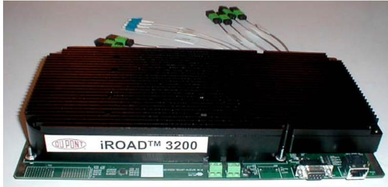
Fig. 4. SSA-based Gen 1 Type I ROADM subsystem with optical connectors on a line card with electrical connectors.
