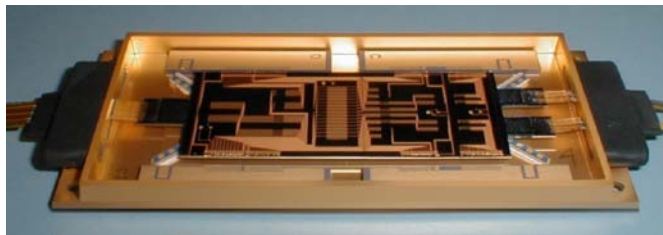
Fig. 14. 8 \times 8 matrix switch with power monitoring and automatic power balancing.
