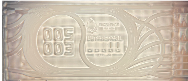
Figure 3. Photograph of a 4- \lambda LAN-WDM multiplexer chip, fabricated in silica-on-silicon with a refractive index contrast of \Delta n = 2.0\% and a footprint of 0.15 \text{ cm}^2 .
