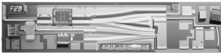
Figure 7. A photograph of a triplexer chip realized by hybrid integration of silica PLC and active components.
